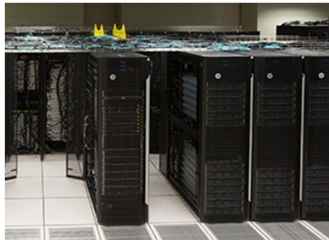
The Bridges supercomputer comprises several refrigerator-sized cabinets, each containing multiple processors.
